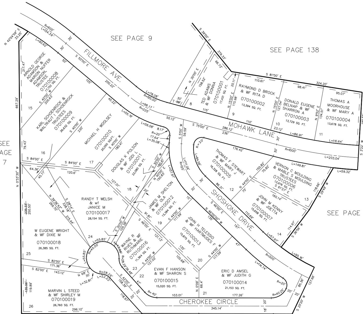
5' UTILITY & DRAINAGE EASEMENTS EACH SIDE OF PROPERTY LINES AS INDICATED BY DASHED LINES, EXCEPT AS OTHERWISE SHOWN.
